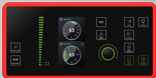
Operator control using light color and light animation.
